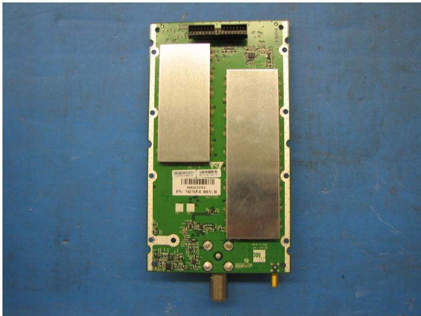
PCB Assembly Bottom View Ant Port with shielding – SRAU
