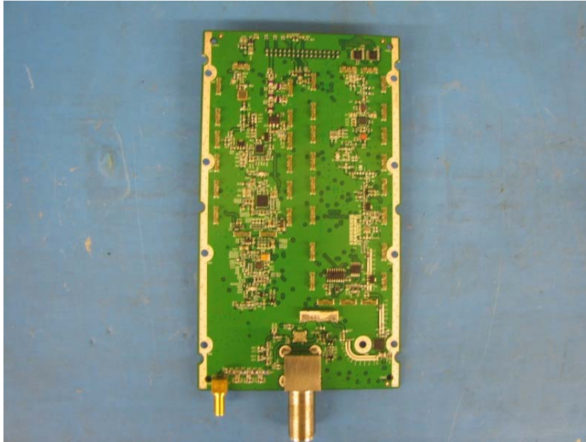
PCB Assembly Top View Ant Port without shielding - SRAU
