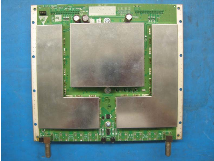
PCB IF Assembly Bottom View with shielding- SRAU
