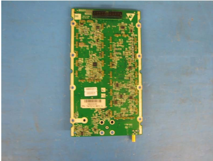
PCB Assembly Bottom View Ant Port without shielding – SRAU
