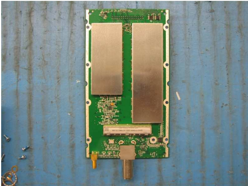
PCB Assembly Top View Ant Port with shielding - MRAU
