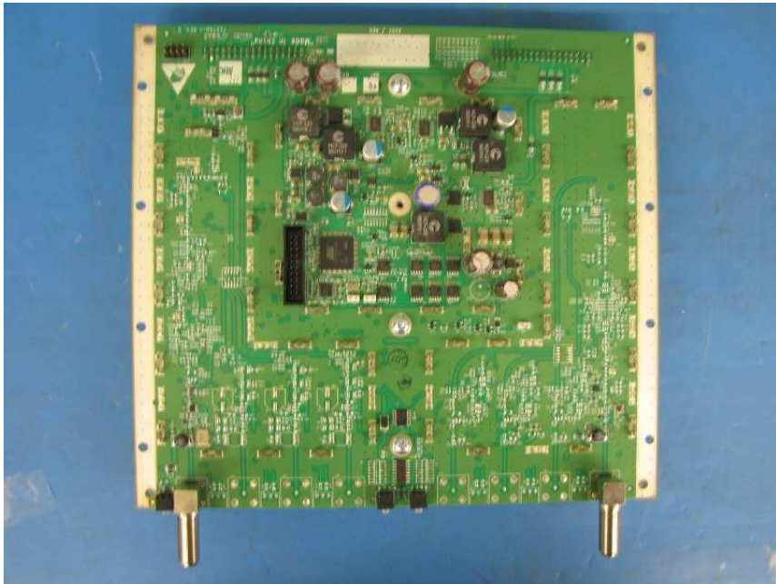
PCB IF Assembly Bottom View without shielding- SRAU
