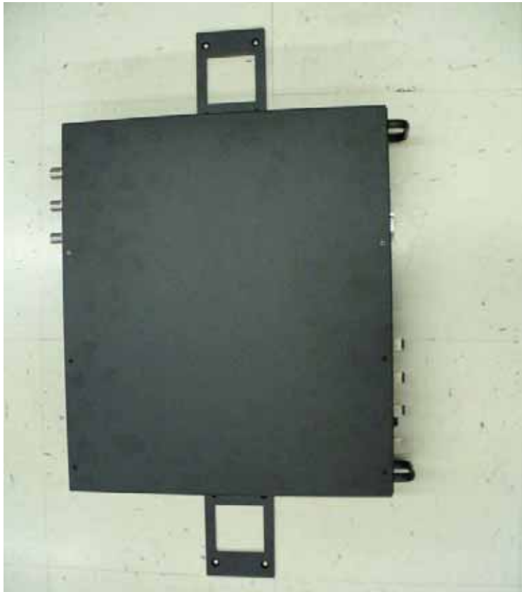
Figure 7-3 Installing Directly to the Wall
