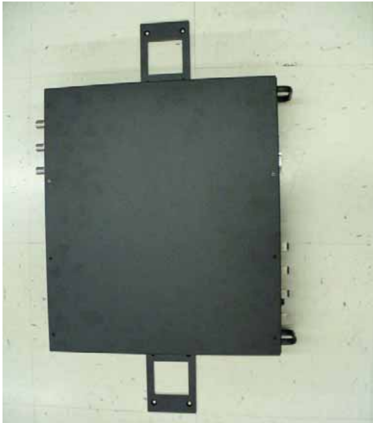
Figure 7-18 Installing Directly to the Wall
