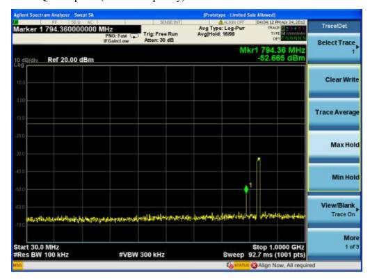
Cellular-LTE-16QAM uplink(middle frequency) Above 1GHz
