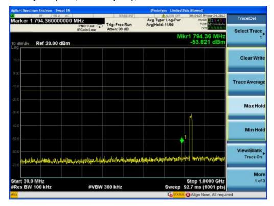
Cellular-LTE-64QAM uplink(middle frequency) Above 1GHz
