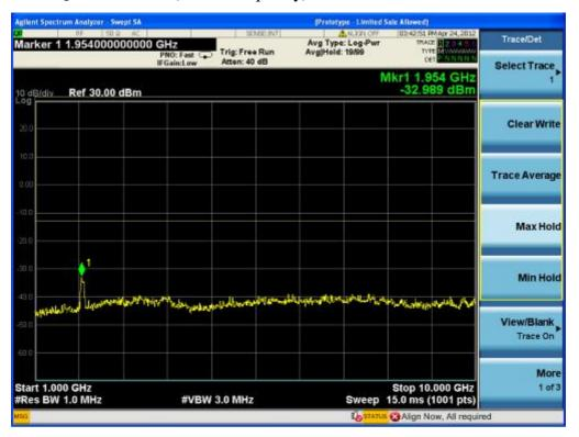
Cellular-LTE -64QAM downlink (highest frequency) 30MHz-1GHz
