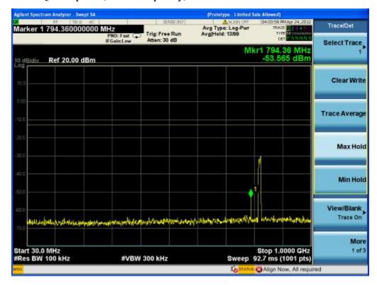
Cellular-LTE-64QAM uplink (lowest frequency) Above 1GHz
