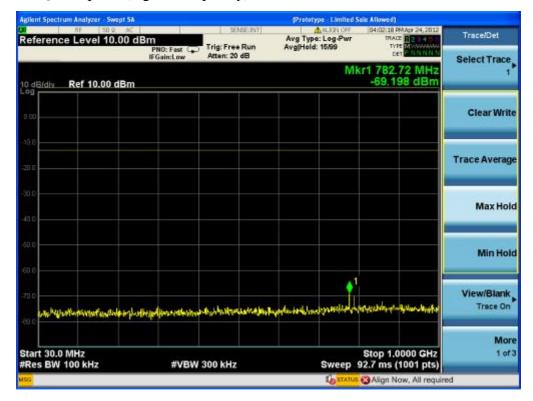
PCS -LTE-16QAM uplink (highest frequency) Above 1GHz
