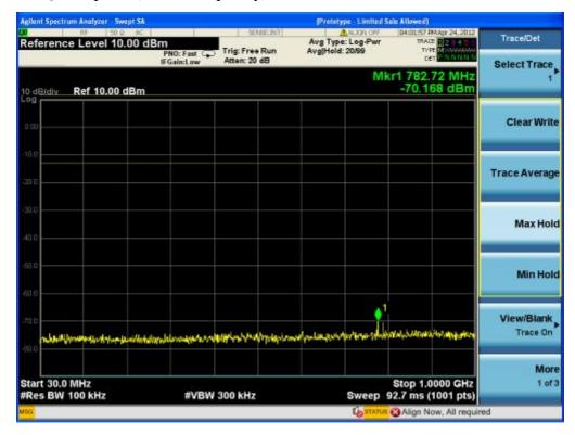
PCS -LTE-64QAM uplink(middle frequency) Above 1GHz
