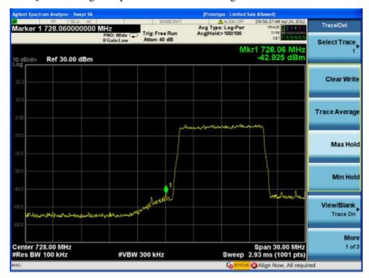
700MHz- LTE-QPSK one signal input down link-Upper Edge
