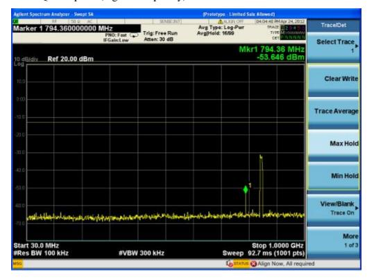
Cellular-LTE-16QAM uplink (highest frequency) Above 1GHz
