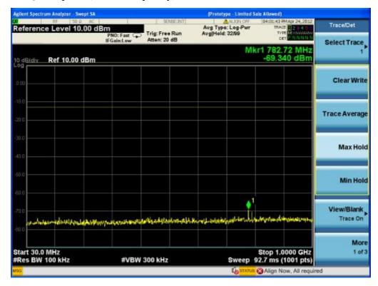
PCS -LTE-16QAM uplink(middle frequency) Above 1GHz
