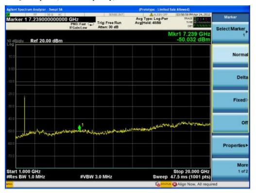
PCS -LTE-16QAM uplink (highest frequency) 30MHz-1GHz
