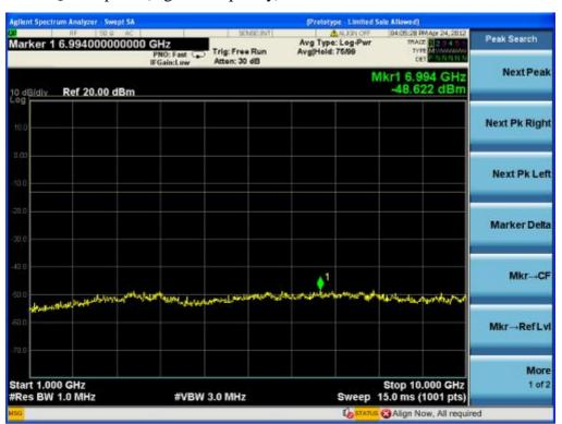
Cellular-LTE-64QAM downlink (lowest frequency) 30MHz-1GHz
