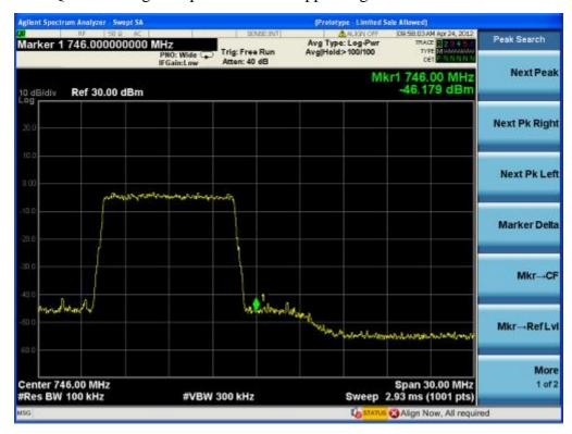
700MHz-LTE-16QAM one signal input down link-Lower Edge
