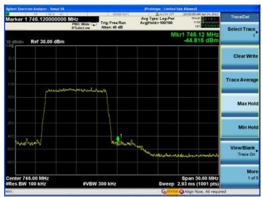
700MHz-LTE-64QAM one signal input down link-Lower Edge
