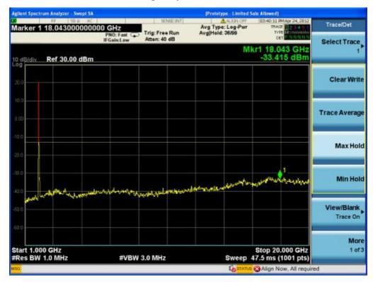
PCS -LTE-16QAM downlink (middle frequency) 30MHz-1GHz
