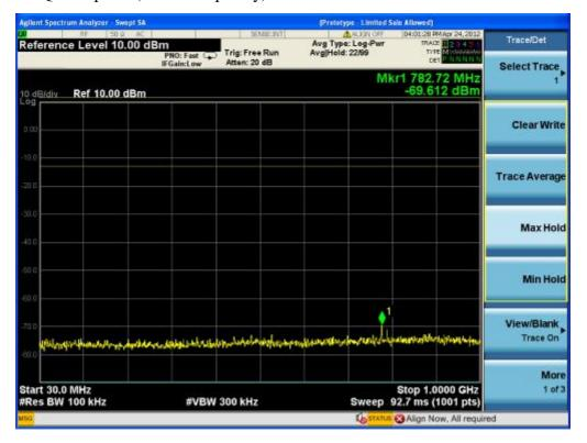
PCS -LTE-64QAM uplink (lowest frequency) Above 1GHz
