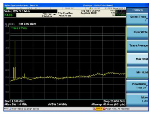
PCS -LTE-QPSK uplink (middle frequency) 30MHz-1GHz
