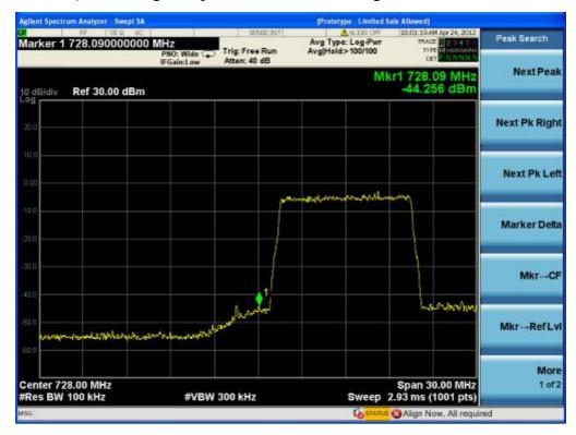
700MHz- LTE-16QAM one signal input down link-Upper Edge
