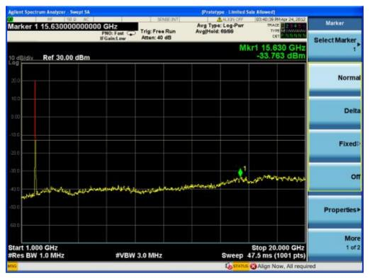
PCS -LTE-64QAM downlink (middle frequency) 30MHz-1GHz
