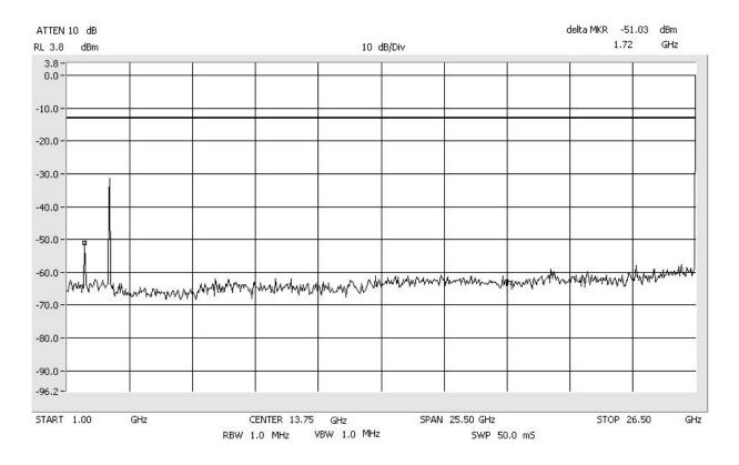
Intermodulation QPSK\_Low\_High WiMAX Center: 2675 MHz Span: 60 MHz RBW/VBW: 100 kHz
