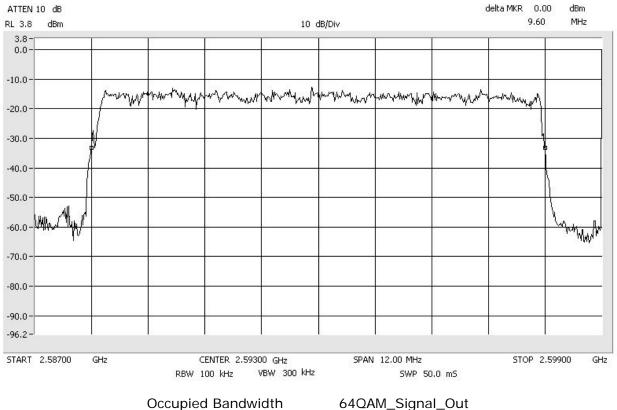
Span: 12 MHz RBW: 100 kHz VBW: 300 kHz
