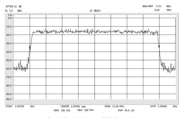
Occupied Bandwidth QPSK\_Signal\_Out Span: 12 MHz RBW: 100 kHz VBW: 300 kHz
