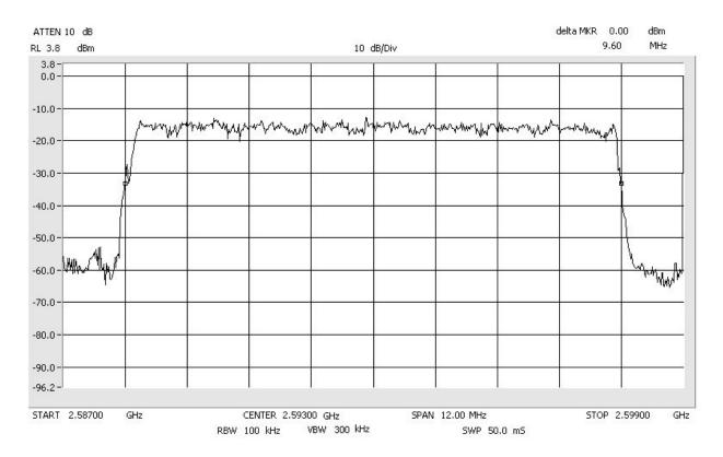
Occupied Bandwidth 64QAM\_Signal\_Out Span: 12 MHz RBW: 100 kHz VBW: 300 kHz
