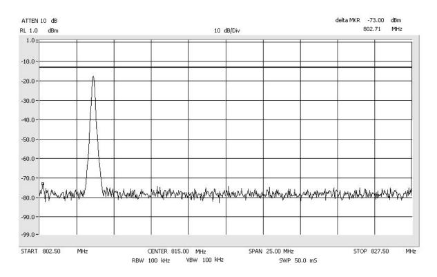
Conducted Emissions Low SMR\_800\_MHz Span: 30 MHz to 10 GHz RBW/VBW: 1 MHz
