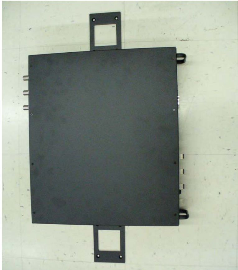
Figure 7-18 Installing Directly to the Wall
