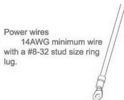
Figure 7-12 Power Wires and Studs
