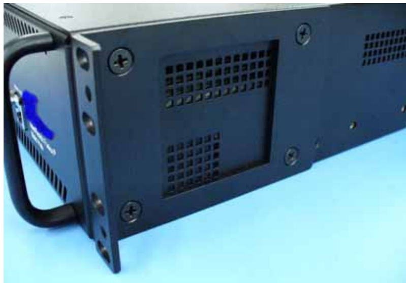
Figure 7-1 Flush Mounting Bracket Detail
