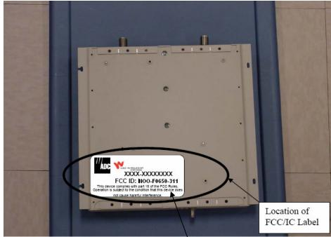
This device complies with part 15 of the FCC Rules. Operation is subject to the condition that this device does not cause harmful interference.
