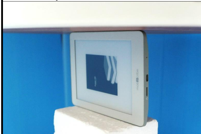
Body - Right Side of EUT at 0 mm
