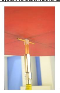
Construction: Symmetrical dipole with 1/4 balun **Enables**
