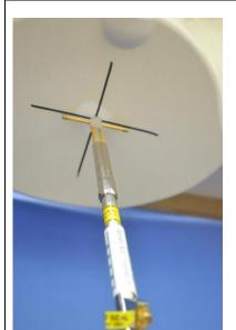
Construction: Symmetrical dipole with 1/4
