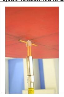
Construction: Symmetrical dipole with 1/4 balun **Enables**
