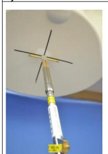
Construction: Symmetrical dipole
