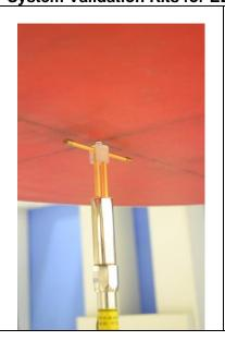
Construction: Symmetrical dipole with 1/4 balun **Enables**
