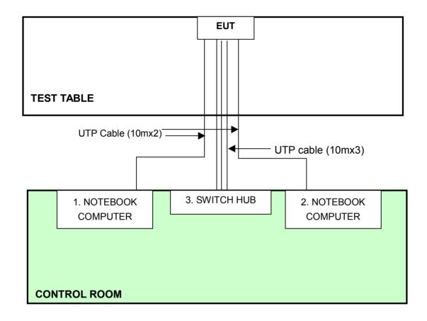
**NOTE:** 1. Support unit  $1 \sim 3$  were kept in the control room during the test.
