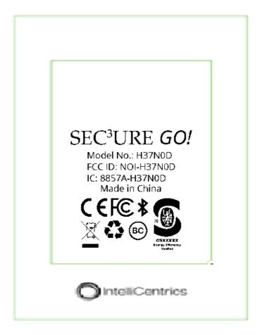
The e-label information is shown on device EPD screen by factory default. To access the e-label information during user operation, press the power button of the device five times.
