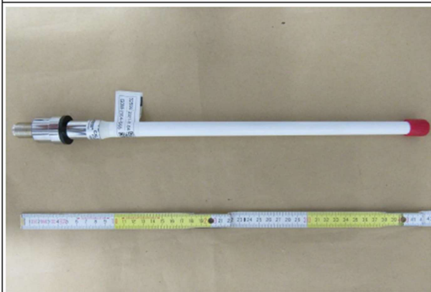
Antenna \lambda/2 dipole CXL 900-1
