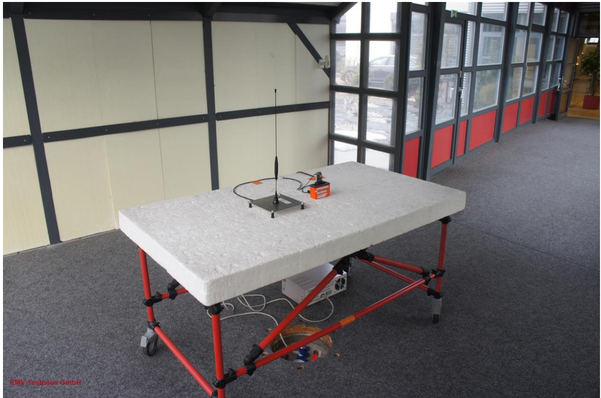
Picture 3: Test setup radiated emission at OATS, front view
