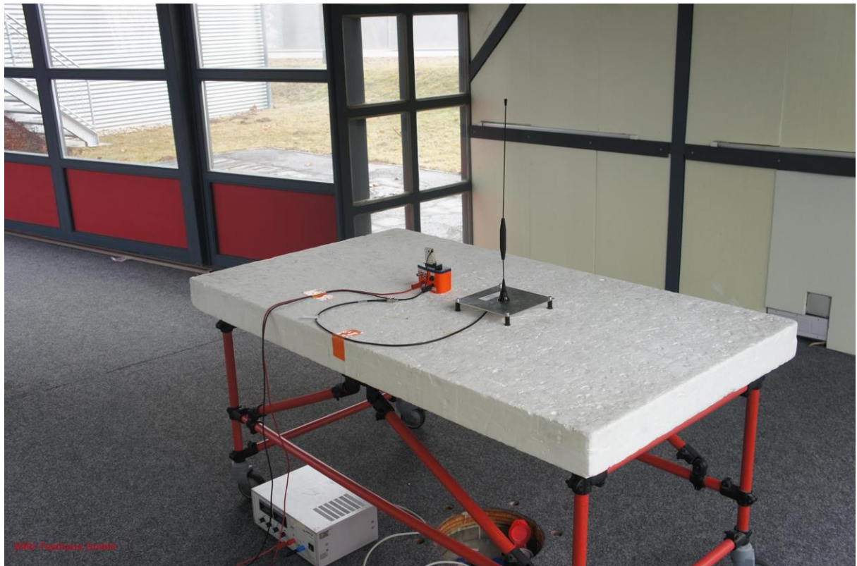
Picture 4: Test setup radiated emission at OATS, rear view
