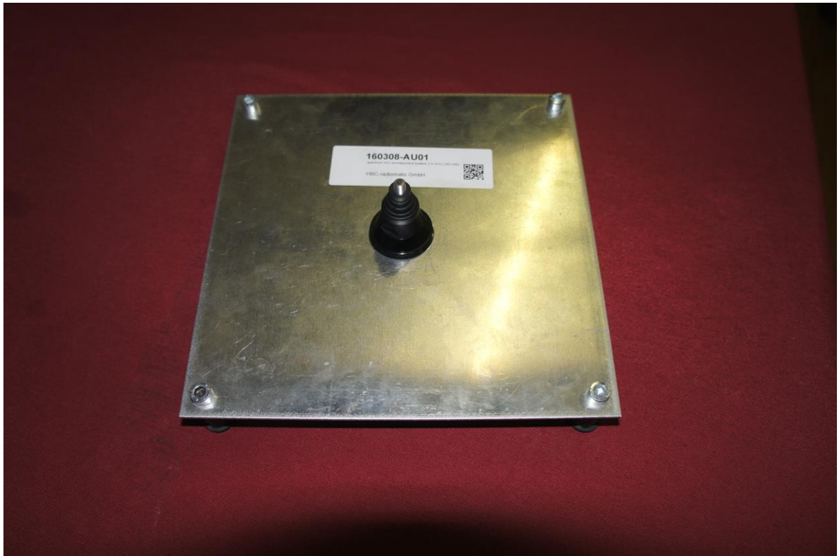
Picture 9: Antenna reference plane - top side
