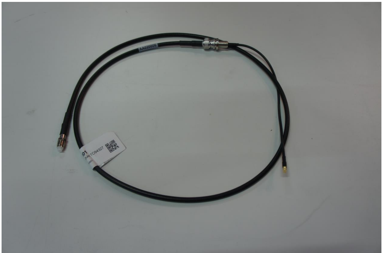
Picture 8: EUT - antenna cable MMCX <-> FME
