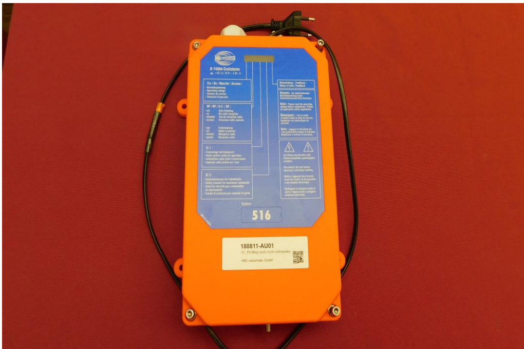
Picture 14: Companion device for RF exposure and EUT for AC powerline measurement
