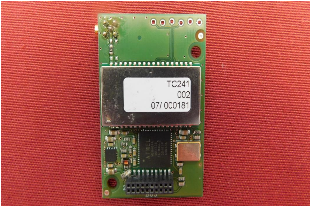
Picture 1: Top view of EUT with host interface TC20 with antenna connector
