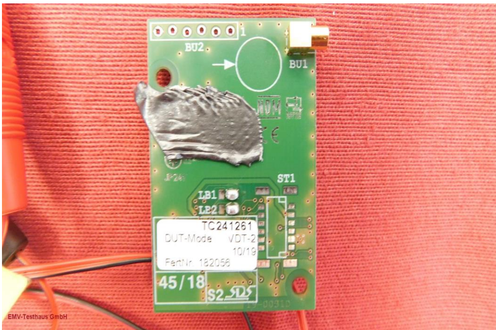
Picture 2: Back view of EUT with host interface TC20 with antenna connector
