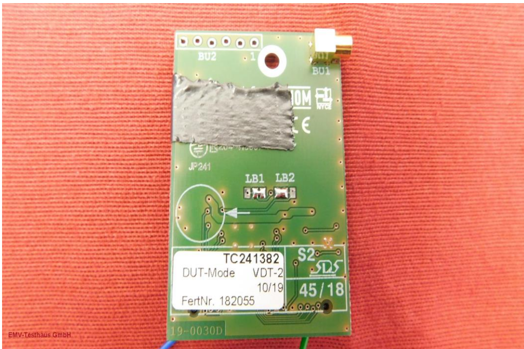
Picture 4: Back view of EUT with host interface TC38 with antenna connector
