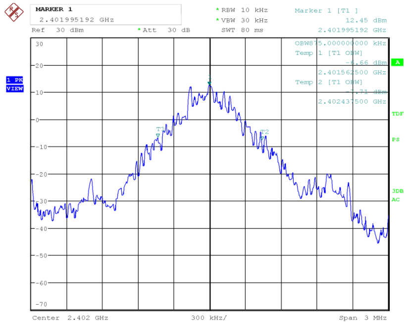
Figure 17: Chart of occupied bandwidth test on channel low (GFSK, DH1)
