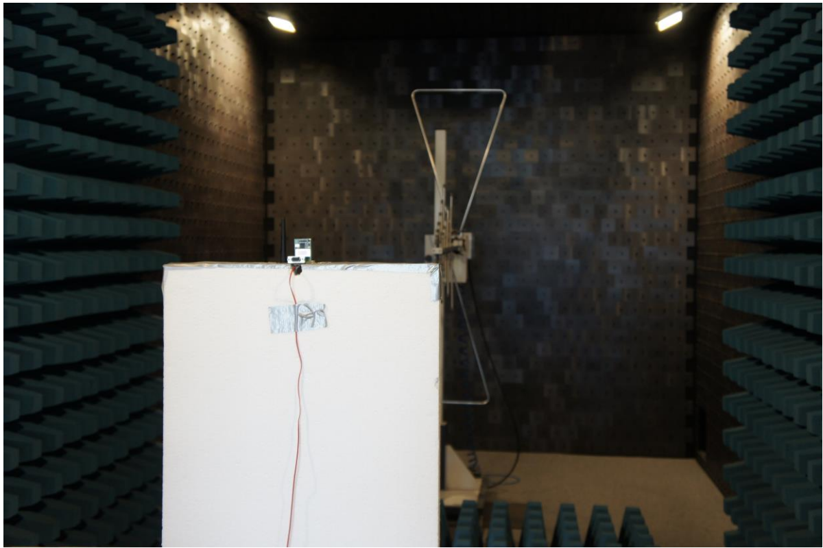
Picture 5: EUT test setup radiated emission test 30 MHz - 1 GHz
