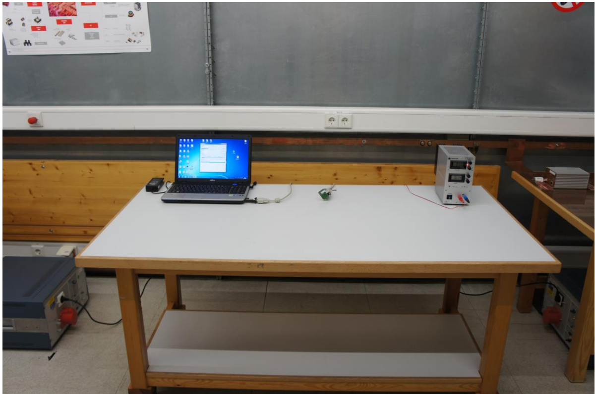
Picture 1: EUT test setup AC power line conducted emissions (front view)
