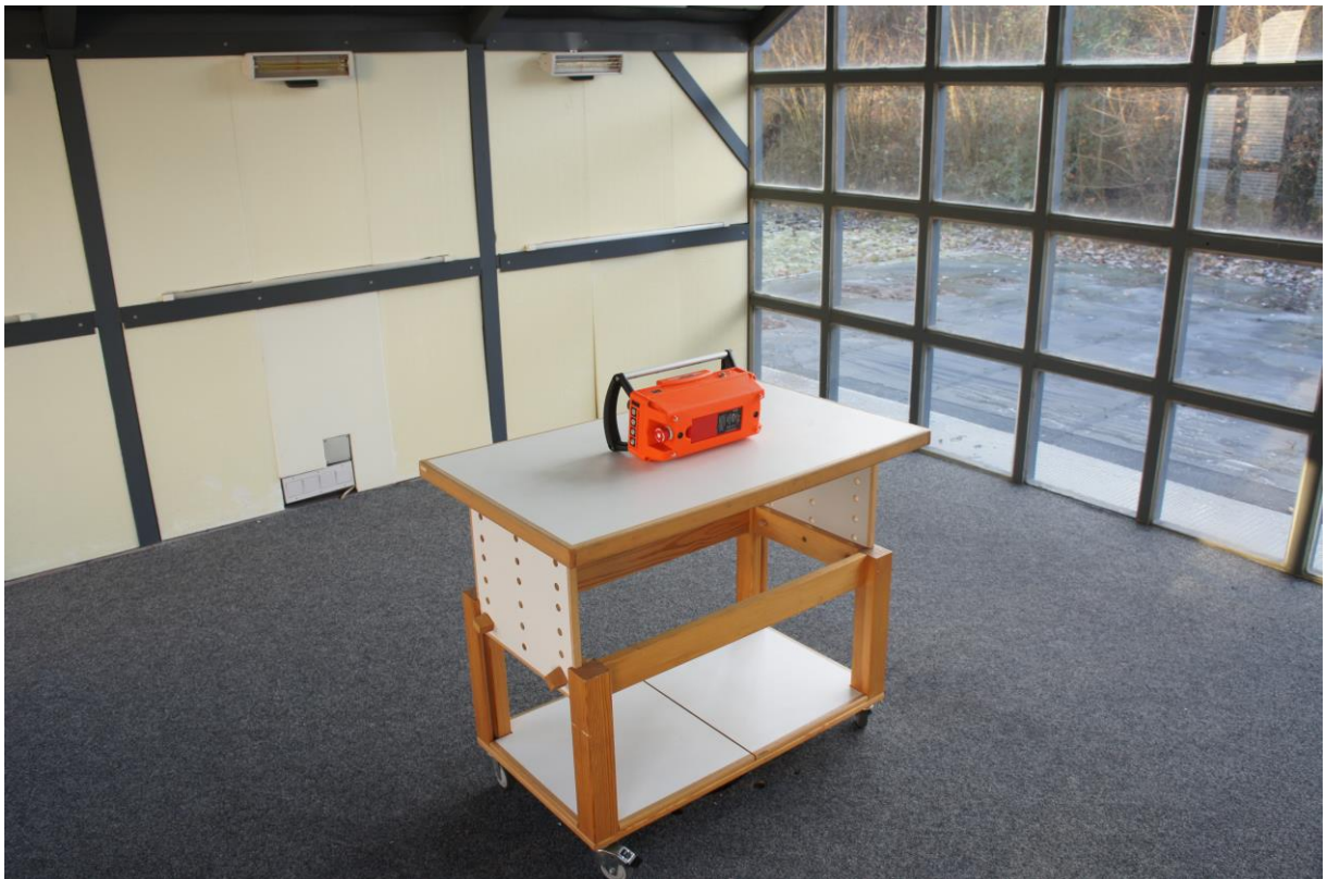
Picture 5: OATS, test setup final radiated emission test < 1 GHz (rear view)
