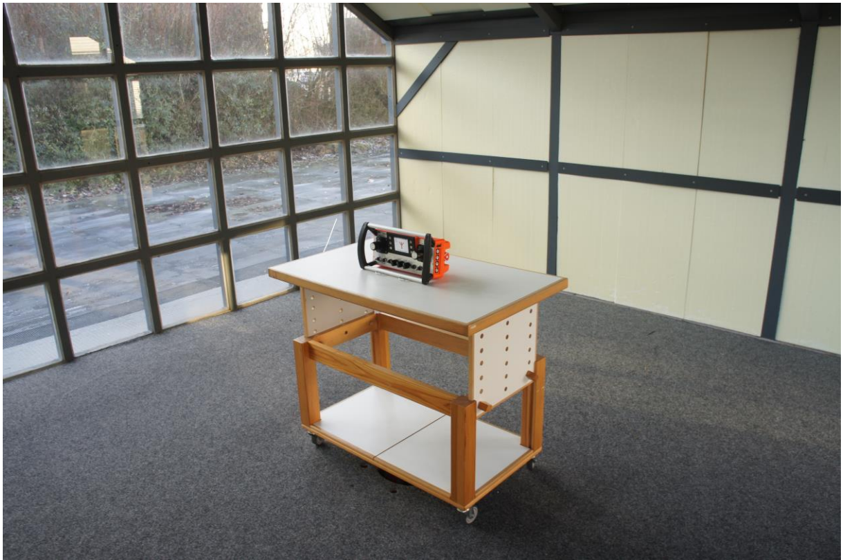
Picture 4: OATS, test setup final radiated emission test < 1 GHz (front view)
