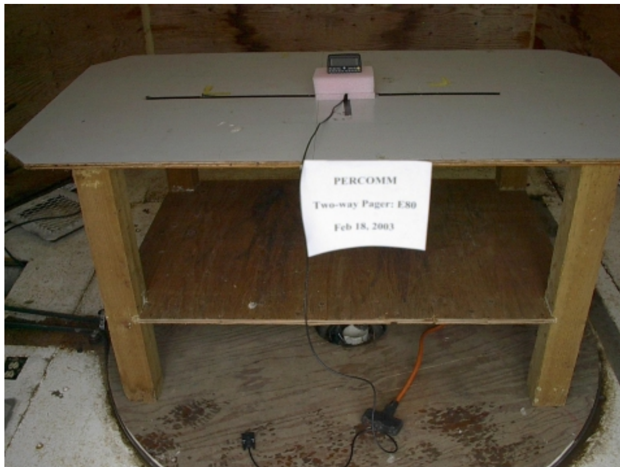
Emissions Test Setup front View (Pager with Serial Cable)
