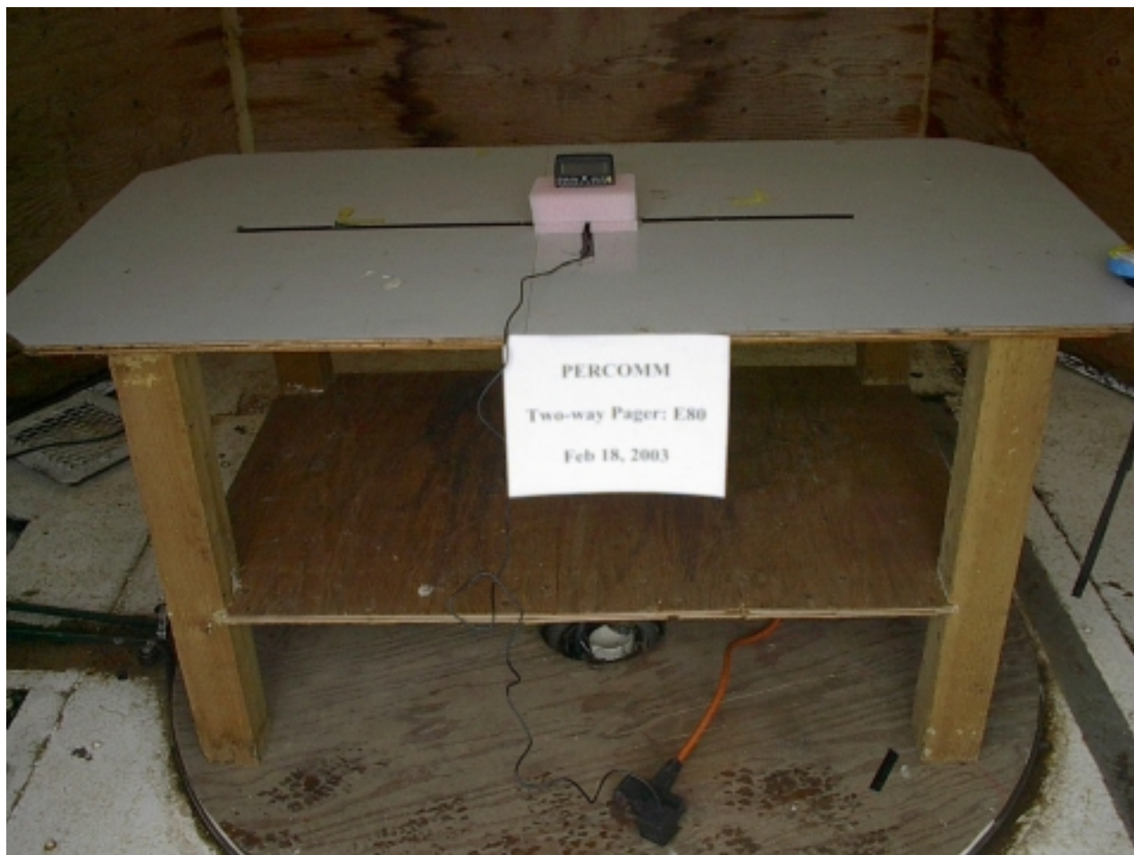
Emissions Test Setup front View (Pager with Power Supply)
