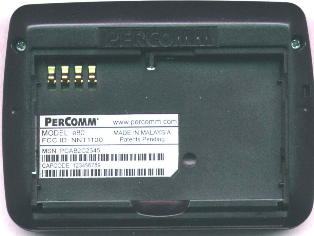
FCC ID Marking is printed on a label placed inside the battery compartment.
