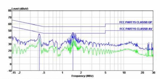
Condition : FCC PART15 CLASSB QP LISN(2011) LINE EUT : RFID Reader Model : SAAT-F805 Test Mode : Standby Power Rating : AC 120V/60Hz Test Engineer: David
