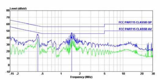
Condition : FCC PART15 CLASSB QP LISN(2011) NEUTRAL EUT : RFID Reader Model : SAAT-F805
