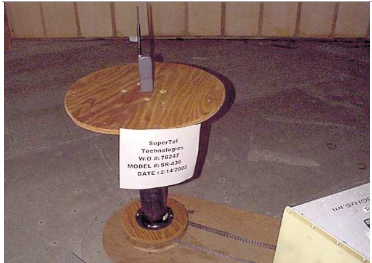
Radiated Emissions - Back View - SR-436 Handset Vertical
