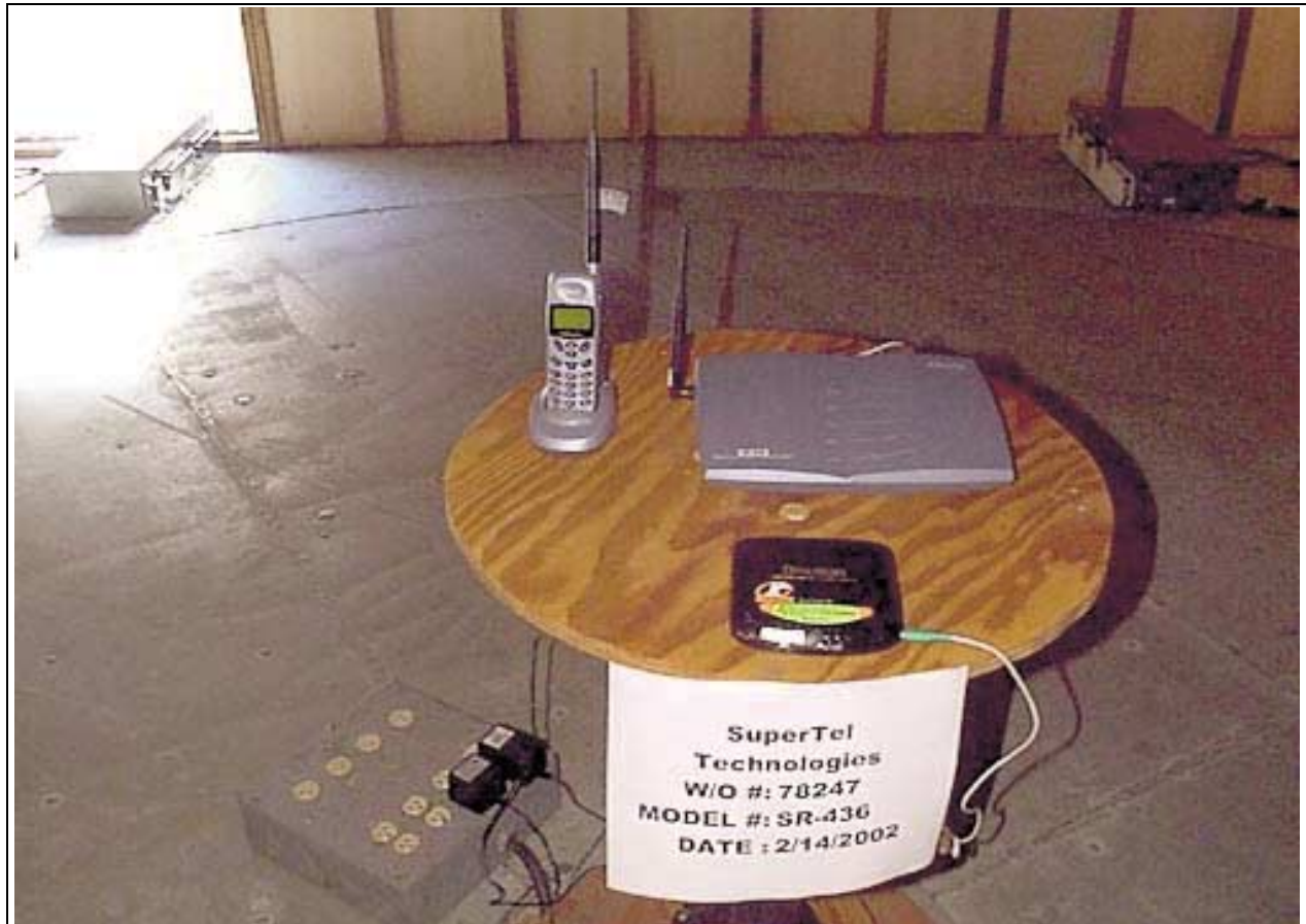
Radiated Emissions - Front View - SR-436 Base and Charger
