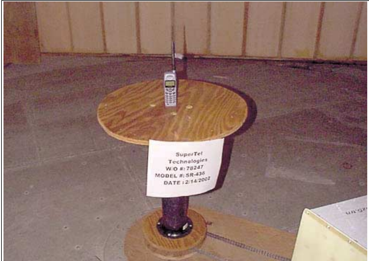
Radiated Emissions - Front View - SR-436 Handset Vertical
