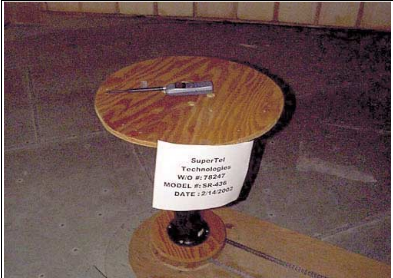
Radiated Emissions - Front View - SR-436 Handset Horizontal
