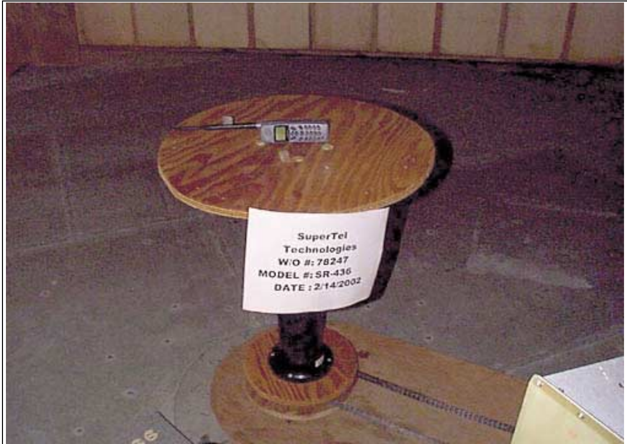
Radiated Emissions - Back View - SR-436 Handset Side
