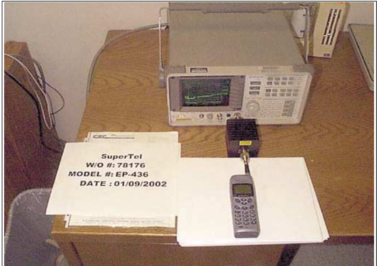
Antenna Conducted - Handset
