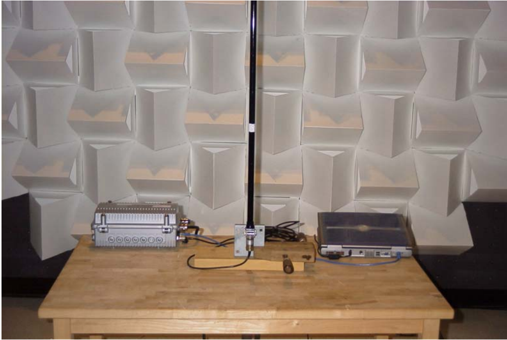
Radiated Emission Test Setup – YA2418RD Antenna
