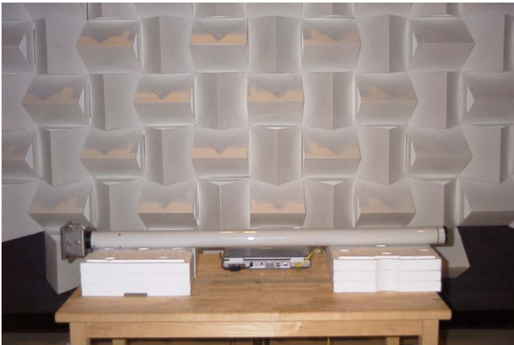
Radiated Emission Test Setup – YA2418RD Antenna
