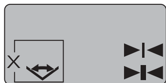
Level laser, Line Dither/Scan mode, Detector off
