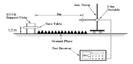
The radiated emission tests were performed in the 3 meters test site, using the setup accordance with the ANSI C63.10-2013. The specification used was the FCC 15  $\S$  15.209, 15.205 and 15.231.
