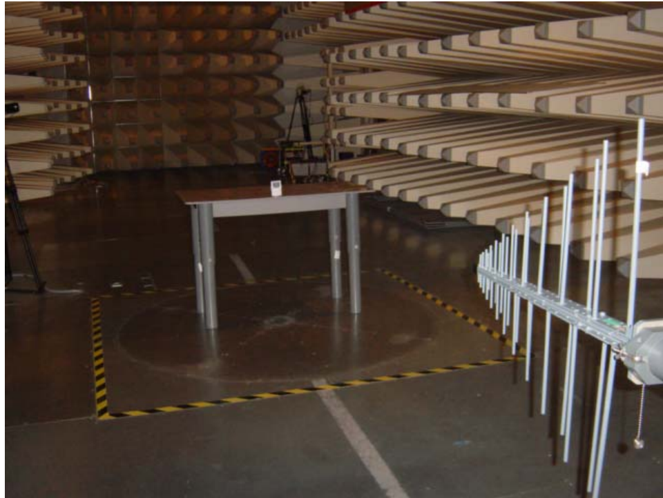
Set-up for Radiation Emission (Transmitter)
