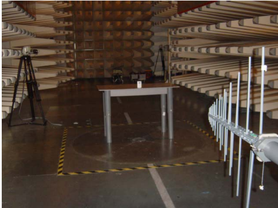
Set-up for Radiation Emission (Transmitter)
