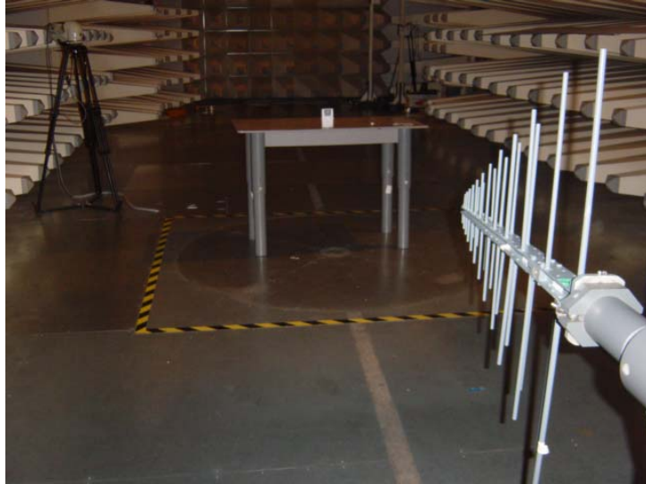
Set-up for Radiated Emission (Transmitter)
