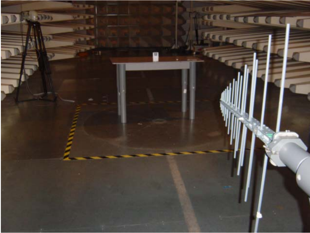
Set-up for Radiation Emission ( Transmitter)
