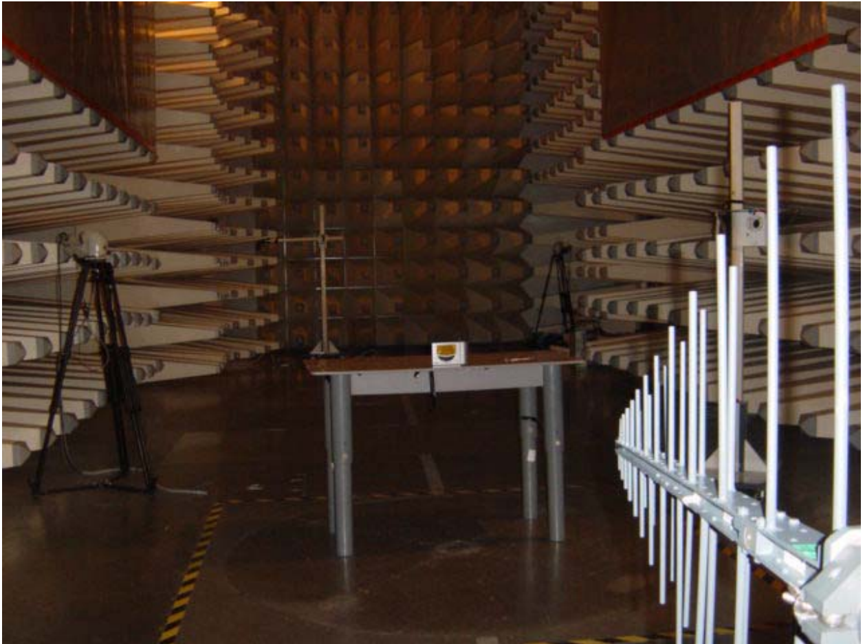
Set-up for Radiation Emission (Transmitter)
