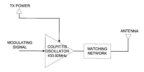
BWR10X **Trasmitter Module Block Diagram**
