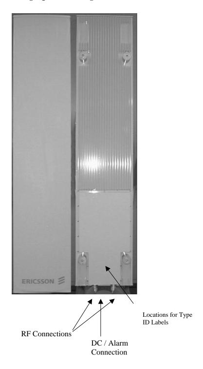
Figure 8-1 Photographs of the Active Antenna Assembly
