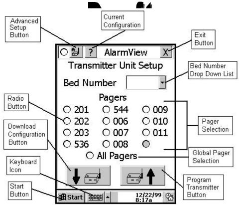
To obtain the current configuration programmed into the transmitter, tap the "Download Configuration Button". When this button is tapped, the PDA attempts to establish communications with the transmitter. If the IR port could not be accessed, the following dialog box will be displayed.
