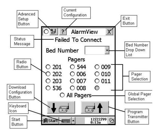
At this point, simply point the PDA at the transmitter, and tap the "Download Configuration Button" again. While the transmitter is being queried, the Configuration Program main screen will be displayed with a status message informing the user of a "Loading Data" status. The PDA will be in this state for less than 2 seconds.
