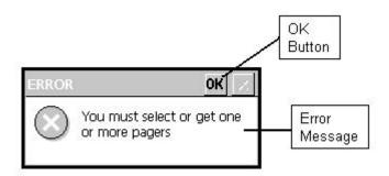
Exit both of the above dialog boxes by tapping the OK Button. After the above error conditions are rectified, tap the "Program Transmitter" button again. When this button is tapped, the PDA attempts to establish communications with the transmitter.
