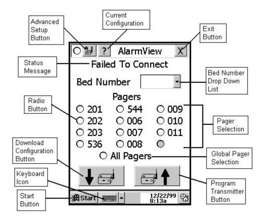
At this point, simply point the PDA at the transmitter, and tap the "Program Transmitter Button" again. While the transmitter is being queried, the Configuration Program main screen will be displayed with a status message informing the user of a "Programming" status. The PDA will be in this state for less than 2 seconds.
