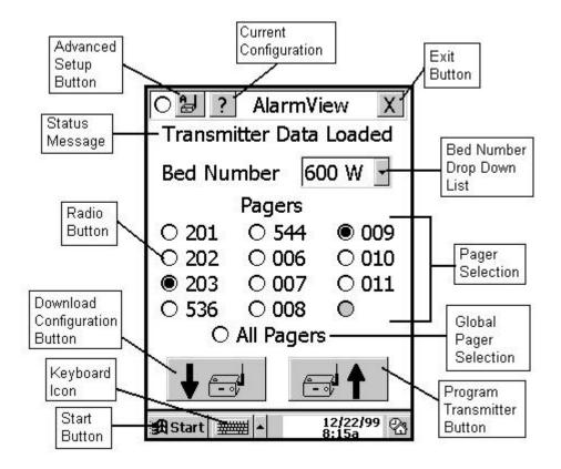
At this point, if the displayed data is correct, no changes need be made, and the user is done. Exit the Configuration Program by tapping the "X" in the upper right corner of the screen.
