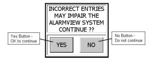
Pressing the "No Button" will return the user to the AlarmView System Manager main screen. Pressing the "Yes Button" will launch the "AlarmView Editor" program. This is the program used to setup which bed number and cap codes are present in the system. It can be reconfigured when pagers are sent back to the factory, or new pagers are obtained.
