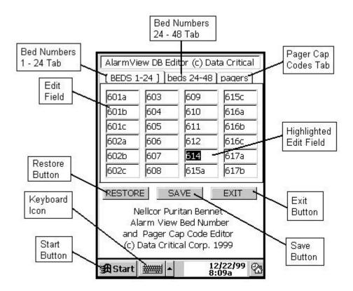
If the key board is not visible, tap the keyboard icon to display the keyboard. If an additional bed number is desired, a bed number can be added to any blank space on page one or two of the bed number listing. Simply tap the cursor in the blank space and begin typing the new bed number.
