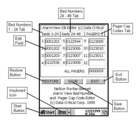
Pager Cap Codes can be added and deleted from this list. Click on a cap code number to edit. Using the stylus, tap the backspace key on the keyboard to delete the cap code number to be edited (or highlight the entire cap code number), and using the numbers and letters on the key board, type in the new cap code number. Tap the "Save" button on completion, or the "Exit" button to exit the Editor Program.
