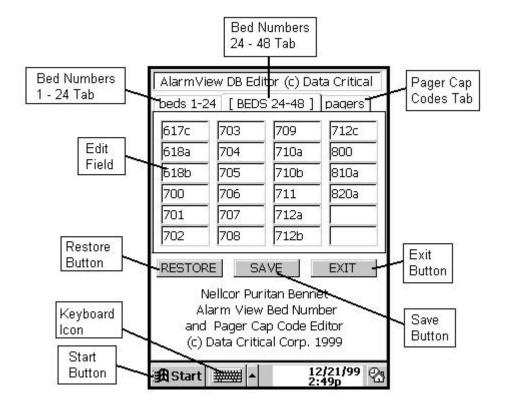
Bed Numbers can be added and deleted from this list. Click on a bed number to edit. Using the stylus, tap the backspace key on the keyboard to delete the bed number to be edited (or highlight the entire bed number as shown below), and using the numbers and letters on the key board, type in the new bed number. Tap the "Save" button on completion, or the "Exit" button to exit the Editor Program.
