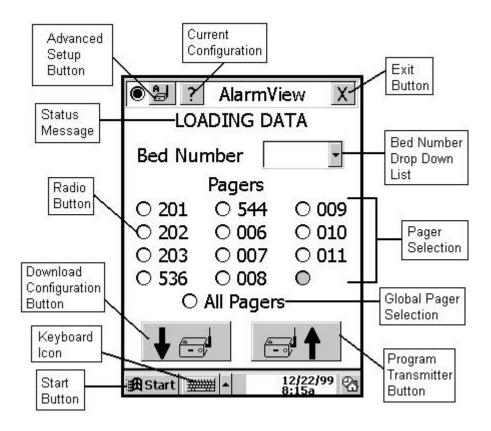
When the transmitter has been successfully queried, the Configuration program main screen will be displayed with a status message informing the user of a "Transmitter Data Loaded" status.
