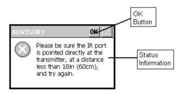
When "OK" is tapped on this dialog box, the Configuration Program main screen will be displayed with a status message informing the user of a "Failed to Connect" status.
