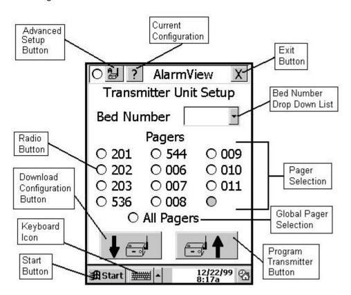
To obtain the current configuration programmed into the transmitter, tap the "Download Configuration Button". When this button is tapped, the PDA attempts to establish communications with the transmitter. If the IR port could not be accessed, the following dialog box will be displayed.
