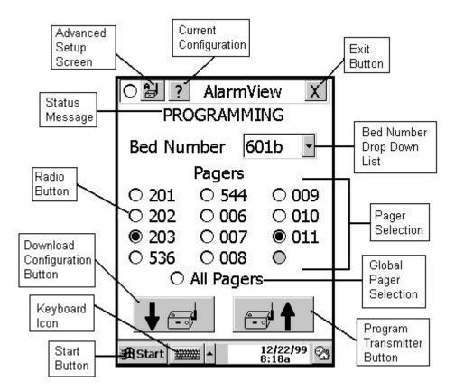
When the transmitter is successfully programmed, the Configuration Program main screen will be displayed with a status message informing the user of a "Programming Successful" status.
