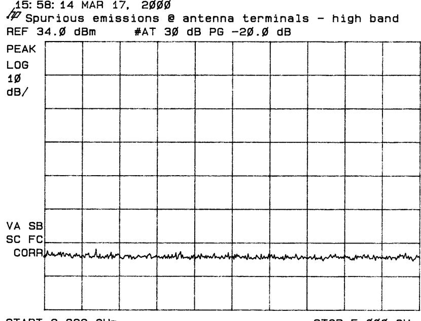
START 2.899 GHz #RES BW 100 kHz #VBW 100 kHz
