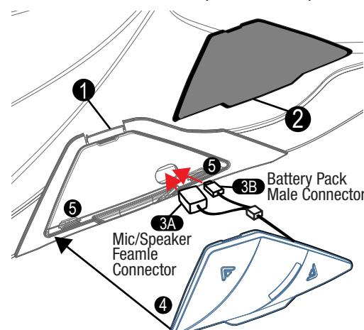
Push up the Locking Lever (1) to remove EXO-COM Controller Cover (2), and put Mic/Speaker Female Connector (3A) into the hole first, and then Battery Pack Male Connector (3B) referring to the above picture.
