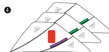
The last unit to pair continues to blink **purple** for 15 secs before system ends the pairing process.
