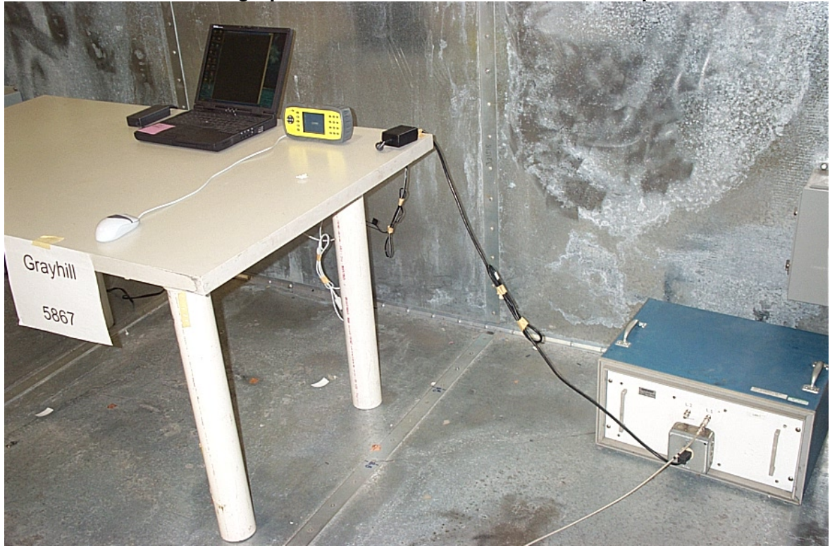
Photograph of Conducted Emissions Test Setup
