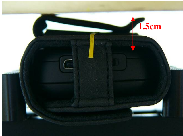
Fig.11 Body worn with Holster 1- EUT front to flat phantom (testing in GPRS Mode), distance between flat phantom and mobile phone is 1.5 cm
