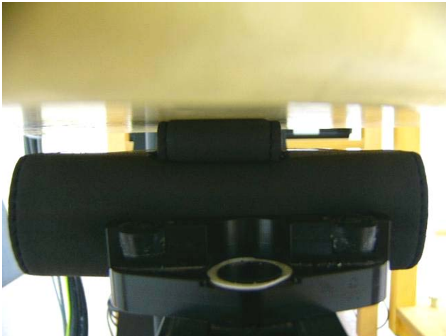
Fig.11 Body worn with Holster 1- EUT front to flat phantom (testing in GPRS Mode), distance between flat phantom and mobile phone is 1.5 cm
