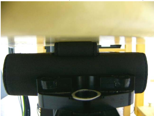
Fig.12 Body worn with Holster 1- EUT back to flat phantom (testing in GPRS Mode), distance between flat phantom and mobile phone is 1.5 cm
