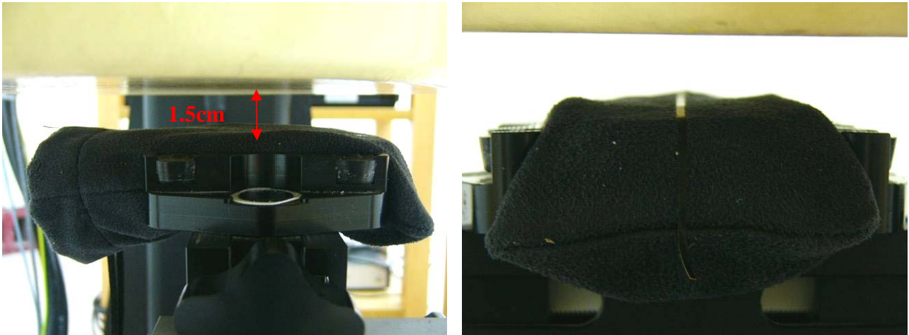
Fig.14 Body worn with Holster2- EUT front to flat phantom (testing in GPRS Mode), distance between flat phantom and mobile phone is 1.5 cm
