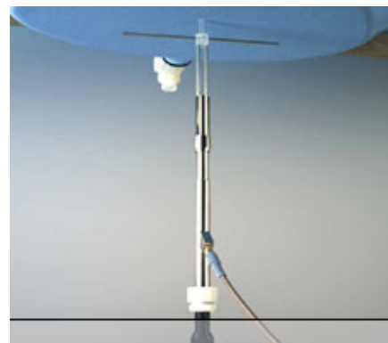
Photograph of the dipole Antenna
